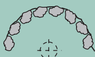
AFTER DRESSING (Wheel face is open with the grits exposed, ready for efficient grinding action.)
