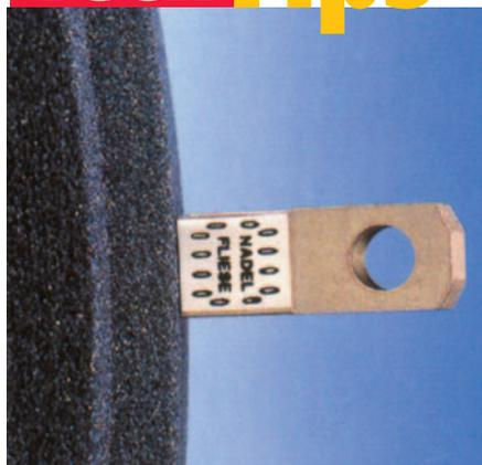
**Carat selection** - The diamond used in the dresser should be large enough so that it has enough surface area to be held well in the shank. Where higher dressing infeeds and traverse rates are required, the carat size of diamond must be higher. Multiply the diameter (in mm) of the wheel by its thickness (in mm). Refer the above value to the chart that follows and select the carat size of diamond. This is a rough method.
